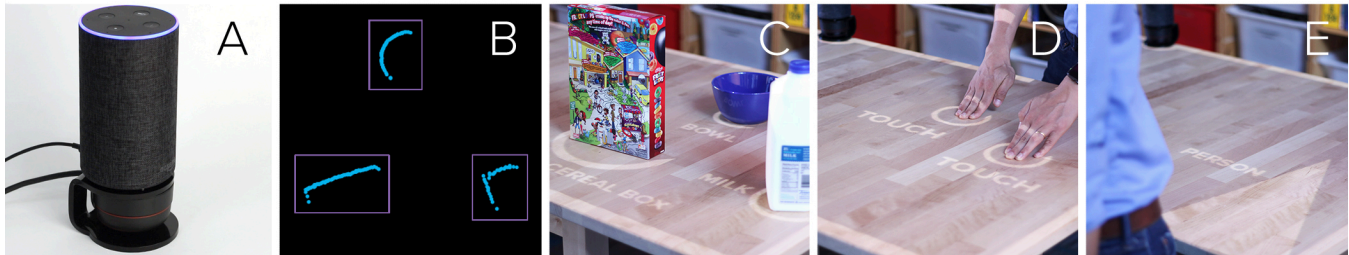
Figure 1. SurfaceSight enriches Internet-of-Things (IoT) experiences with touch, user, and object sensing. This is achieved by adding LIDAR to devices such as smart speakers (A). Next, we perform clustering and tracking (B), which unlocks novel interactive capabilities such as object recognition (C), touch input (D), and person tracking (E).
